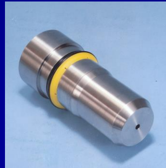
Seal position on Mandrel before belling
