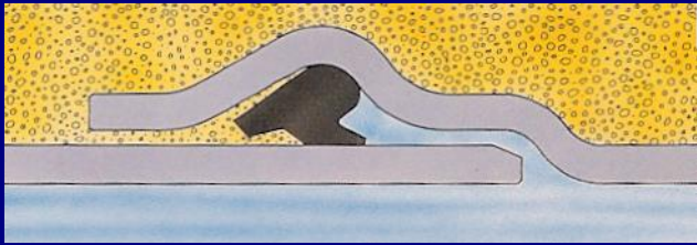
Traditional Seal : Pulsation test under negative pressure. After several pulsations sand ingress starts to wear the seal
